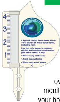
Rain gauges are devices designed to measure how much rain was received at a specific location over a designated period of time. Rain gauges are easy to use and can act as an accurate way to measure how much water plants are getting over time. Use your rain gauge to monitor how much rain was received at your house. Keep track of weekly rainfall totals to determine whether your lawn needs additional water.
